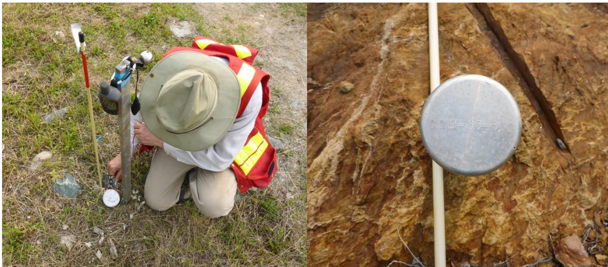
Figure 12.2 GPS and compass checks of Cameron drill collar locations and dip, CCD-11-100 drillhole cap with hole number at deposit outcrop
