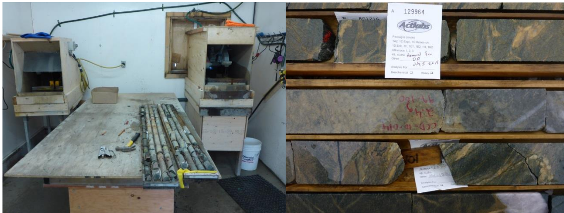
Figure 11.2 Core cutting station and cut core marked up with sampling tickets stapled into the boxes
