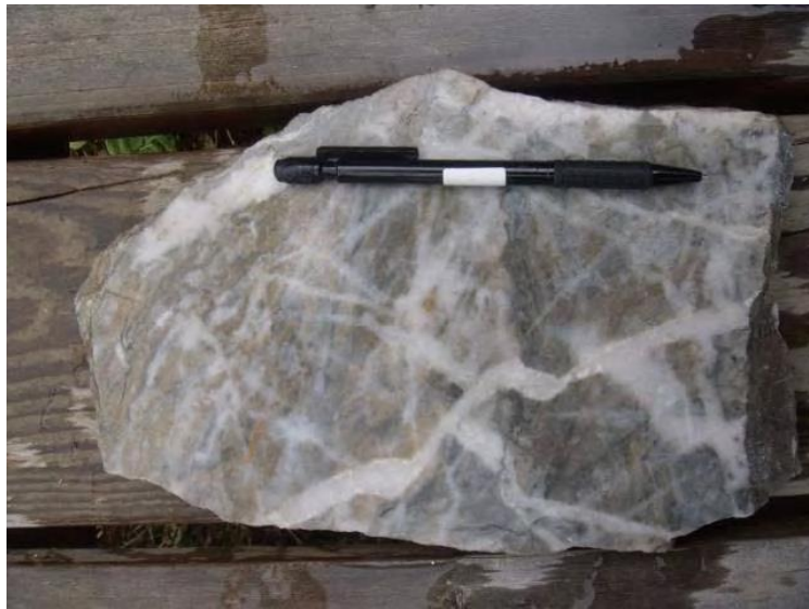
Figure 7.16 Quartz-sulphide stockwork mineralisation from the Cameron Gold Deposit stockpile exhibiting multiple overprinting relationships (Source: Ball, 2014)
